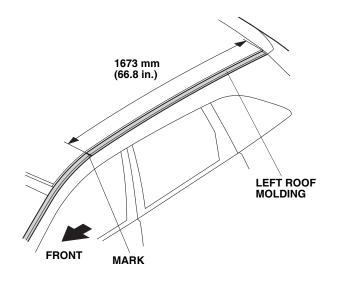
2. Open the tailgate. Using a plastic trim tool, pry up on the left roof molding to release the clip.
