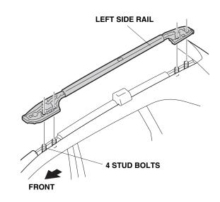
At the left center stay cover, install two TORX screws through the holes in the left side rail. Torque the TORX screws to 7 to 12 N·m (5 to 9 lbf·ft).
