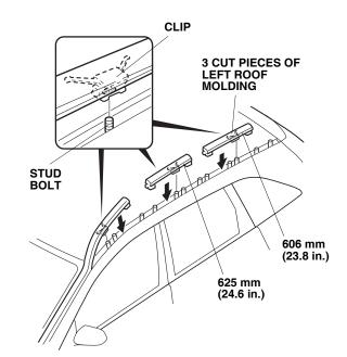
15. Place the left center stay over the two stud bolts at the center, and install two TORX nuts. Torque the TORX nuts to 12 to 15 N·m (9 to 11 lbf·ft).
