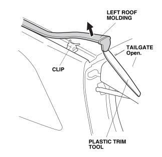
3. Continue to remove the left roof molding by lifting the molding upward to release six more clips. Do not remove the left roof molding along the windshield.
