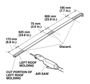
11. While wearing eye protection, use an air saw to cut the left roof molding at the marks you made.
