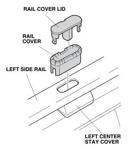
21. Install the rail cover into the hole in the center of the left side rail.
