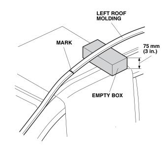
7. While wearing eye protection, cut the left roof molding at the mark using an air saw. Have an assistant hold the rear edge of the left roof molding near the shop towel while cutting.
